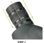
Insert Eyepiece into body
