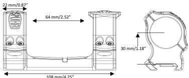
The SCT-4001 Hunting Mount features one Spuhr Interface™ Top Cover, which can be installed as to position any of more than 40 different accessories in either the 12 or 3 o'clock position.
