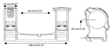
The SCT-3001 Hunting Mount features one Spuhr Interface™ Top Cover, which can be installed as to position any of more than 40 different accessories in either the 12 or 3 o'clock position.
