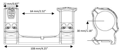
The SCP-4001 Hunting Mount features one Spuhr Interface™ Top Cover, which can be installed as to position any of more than 40 different accessories in either the 12 or 3 o'clock position.
