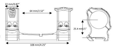
The SCP-3000 Hunting Mount features one Spuhr Interface™ Top Cover, which can be installed as to position any of more than 40 different accessories in either the 12 or 3 o'clock position.
