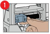
Select applicable Reversible Press Block face and return block to center of Magnum Push Rod.
