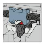
Use this step to ensure everything has remained aligned during the locking process and that the Reversible Press Block remains in correct alignment with the sight or dovetail slot. It must completely clear the slide to prevent damage.
