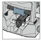
Versatile Slide Cradle accommodates most makes and models of striker-fire and 1911 pistols. Loosen the Spring Loaded Vertical Adjustment Knobs to allow for height clearance and help with visibility. Be sure to check the Hold-Down Clamp, to make sure it is up all the way. Place pistol slide on Slide Cradle.
