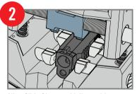
Align Slide Clamp guidelines with center of dovetail slot and secure slide in Slide Cradle.
