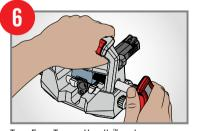
Turn Easy Torque Handle  $^{\mathtt{TM}}$  and push sight through dovetail slot.
