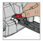
Once the Upper Frame is moved to the correct position, lower the Hold Down Clamp to the top surface of the slide to completely lock slide into place prior to pushing sight.
