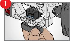
Configure the slide locking base for your Glock model & snugly tighten to hold pistol slide in place.
