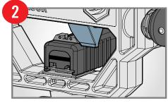
Confirm alignment with Press Block and sight.
