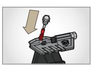
STEP 2. Load spring first, then detent second into the PPT fixture. Compress the spring and detent with the PPT detent plunger and hold.
