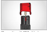
When working with AR10, slide sleeve onto vise block
