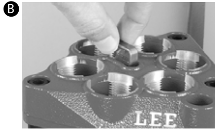
Lower carrier to bottom of the stroke then raise slightly remove index rod.
