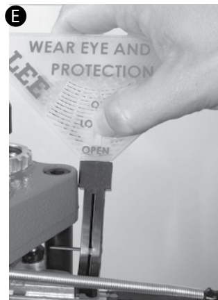
Slide the tray into the trough. Slide the flow control to the ON position.
