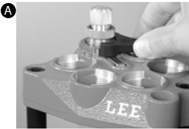
Remove Breech Lock Bushing Die from station 4 to access the index rod.
